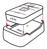
2. The **Battery Indicator** on your Lively Mobile Plus will flash green during the charging process. Once fully charged, the **Battery Indicator** will remain solid green.
