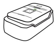
3. To remove your Lively Mobile Plus from the Charging Dock, simply grasp the device and lift it up and away from the Charging Dock. You will hear a tone from the Speaker indicating that it is no longer charging. Unless additional charging is required, the Battery Indicator on the device will turn off to save power.
