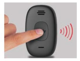
When there is an incoming call, your Lively Mobile2 will ring with an audible tone. Firmly press and release the call button and speak clearly into the microphone located at the bottom of the device.
